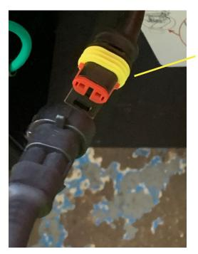
CONNECT REMAINING MULTI PLUG FROM IN FEED TO MAIN BODY.
